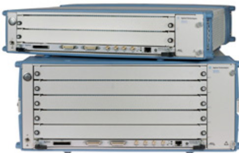
Figure 3 M9502A 2-slot AXIe Chassis and M9505A 5-slot chassis
